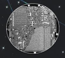
Intel 4004 1<sup>st</sup> Microprocessor 2,300 Transistors
